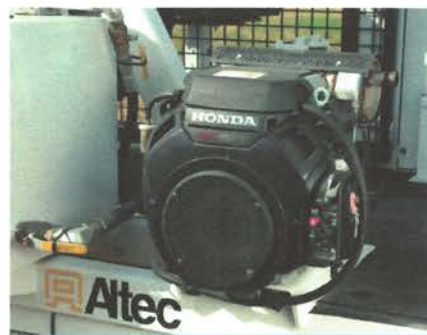
OPTIONAL 22 HP HONDA ENGINE POWERS HYDRAULIC ACCESSORIES
