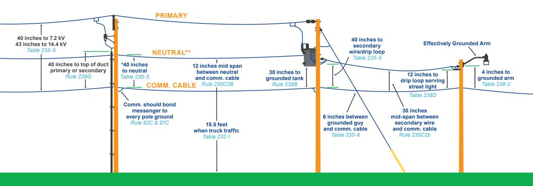
A **communication worker safety zone** is 40 inches of clearance between communication lines and supply lines/equipment per *Rule 235C4 & 238E.*
